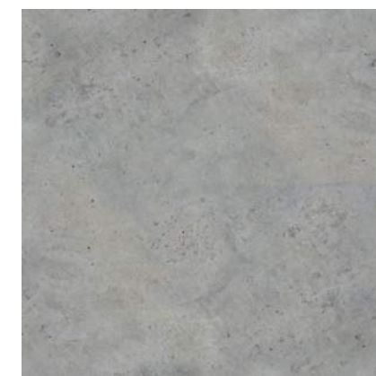
4 SMOOTH 'SACKED FINISH' NATURAL CONCRETE
