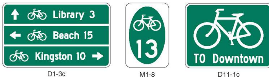
Figure 4-7: Standard CA MUTCD Compliant Bicycle Signage
