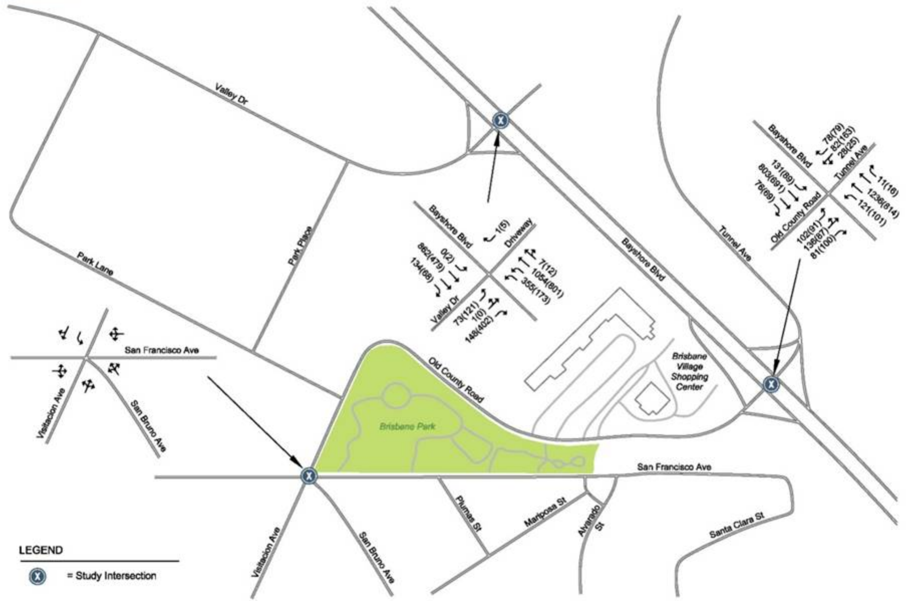
Figure 3 Intersection Lane Geometry & Existing Traffic Volumes
